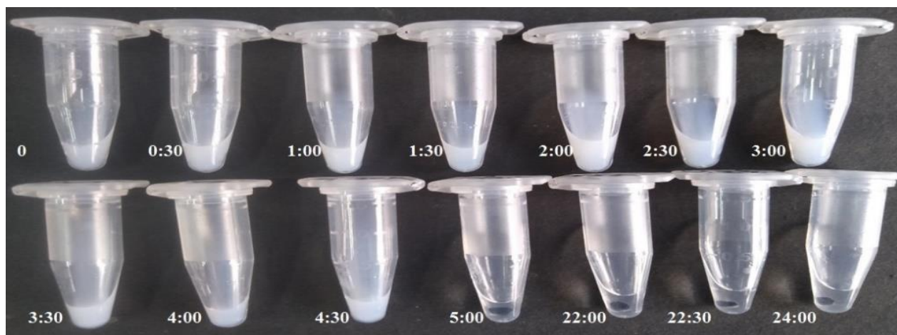
Figure 1 shows the removal of pesticides using biochar at different time points (0-24 hours). Biochar, 10 mg; Chlorpyrifos, 5 mg/mL in Phosphate buffer, pH 7.5
